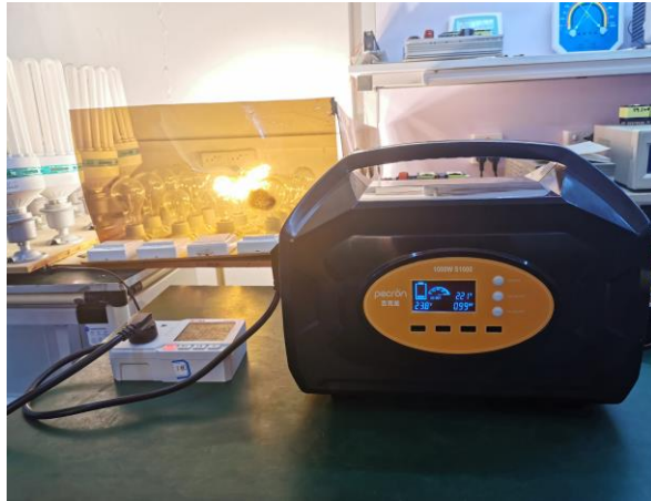
7.2.1 Discharge test under load
